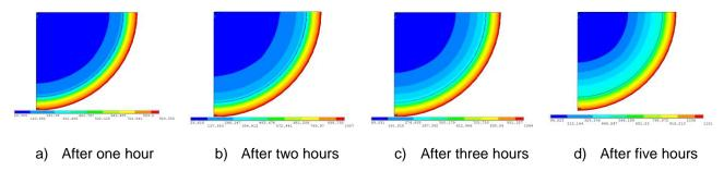
Fig. 25 - Column (1): Numerically predicted temperature distribution in the column cross-section
