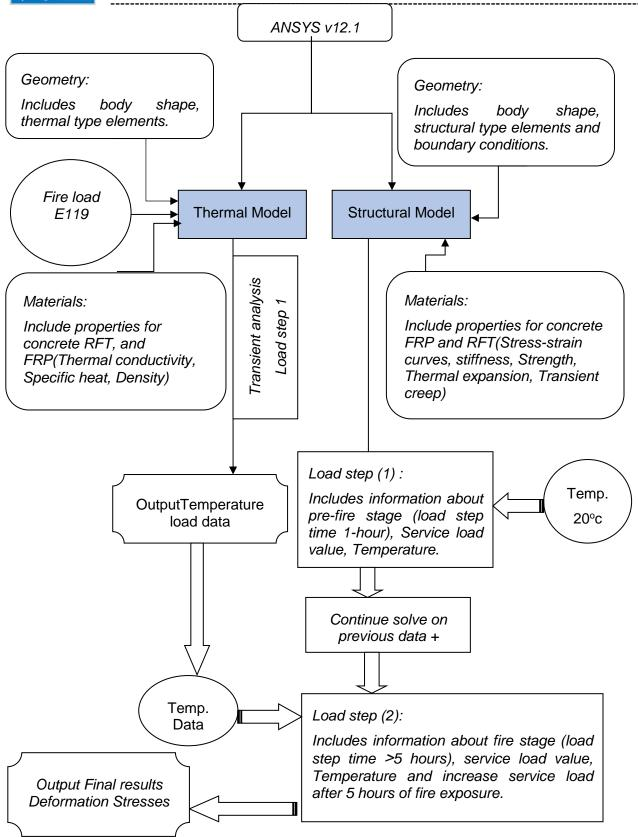
Figure 22: Schematic modeling methodology for RC columns strengthened with FRP
