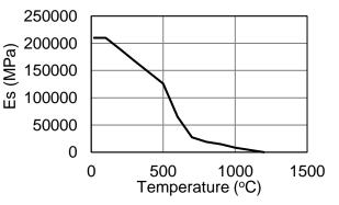
Fig. 11 - Reduction of yield strength of steel with Fig. 12 - Reduction in modulus of elasticity of elevated temperatures [10]
