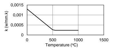
Fig. 5 - Variation of thermal conductivity of typical FRP with elevated temperatures [11]
