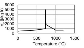
Fig. 6 - Variation of concrete specific heat at elevated temperatures [9]
