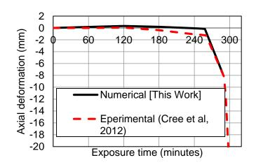
Fig. 33 - Column (4): Axial deformation of the column during fire exposure
