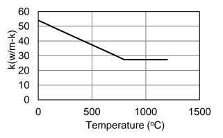
Fig. 4 - Variation of thermal conductivity of steel with temperature [10]
