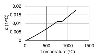
Fig. 16 - Coefficient of thermal expansion of steel with elevated temperatures [10]
